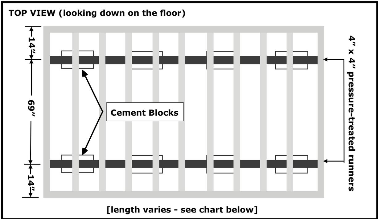
**NOTE:** Measurements are taken from the OUTSIDE of the building to the CENTER of each 4"x 4" pressure-treated floor runner (skid). Runners extend the length of the building.
