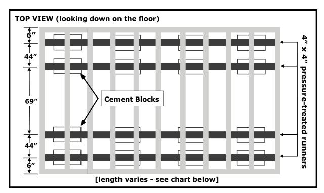
**NOTE:** Measurements are taken from the OUTSIDE of the building to the CENTER of each 4"x 4" pressure-treated floor runner (skid). Runners extend the length of the building.
